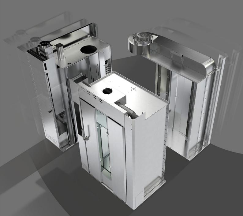
Front side heat exchanger. The oven is made of 1.0 to 4.0 mm gauge stainless steel, while its façade of 1.5 mm gauge sheet steel. The skillful use of different sheet metal gauges and the special bending system employed, plus the exclusive coupling system for individual components, reduce heat losses and optimize heat diffusion. Moreover, since all its parts are fixed with screws, by the constant thermic dilatation, this system is more reliable and guarantees more durability and longevity.
