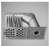
The heat exchanger is where combustion occurs and where the air is heated before coming into contact with the product. The heat exchanger is located on the rear left side of the oven (front left side for the Roller) and it is composed of tubes with the function of increasing the heat exchanger surface area. The combustion gases go through the exchanger (4 turns) untill the chimney exit. The design grants long-lasting working life, by representing the results of experience and know-how.
