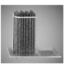
The group of armored tubular finned heating elements is made of AISI 321 stainless steel. Safe and efficient, the elements heat the air to uniform temperature while assuring silent operation and low costs. The heating elements maximize heat exchange and transmit 85% of the heat by convection, rapidly and uniformly, moving large volumes of air. The heating elements are grouped together in areas with individual power feeding lines to allow customized contrai of the consumption/ performance ratio.
