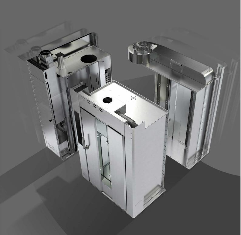
Front side heat exchanger. The oven is made of 1.0 to 4.0 mm gauge stainless steel, while its façade of 1.5 mm gauge sheet steel. The skillful use of different sheet metal gauges and the special bending system employed, plus the exclusive coupling system for individual components, reduce heat losses and optimize heat diffusion. Moreover, since all its parts are fixed with screws, by the constant thermic dilatation, this system is more reliable and guarantees more durability and longevity.
