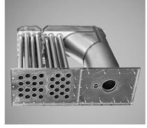
Back side heat exchanger. The oven is made of 1.0 to 4.0 mm gauge stainless steel, while its façade of 1.5 mm gauge sheet steel. The skillful use of different sheet metal gauges and the special bending system employed, plus the exclusive coupling system for individual components, reduce heat losses and optimize heat dispersion. Moreover, since all its parts are fixed with screws, by the constant thermic dilatation, this system is more reliable and guarantees more durability and longevity.
